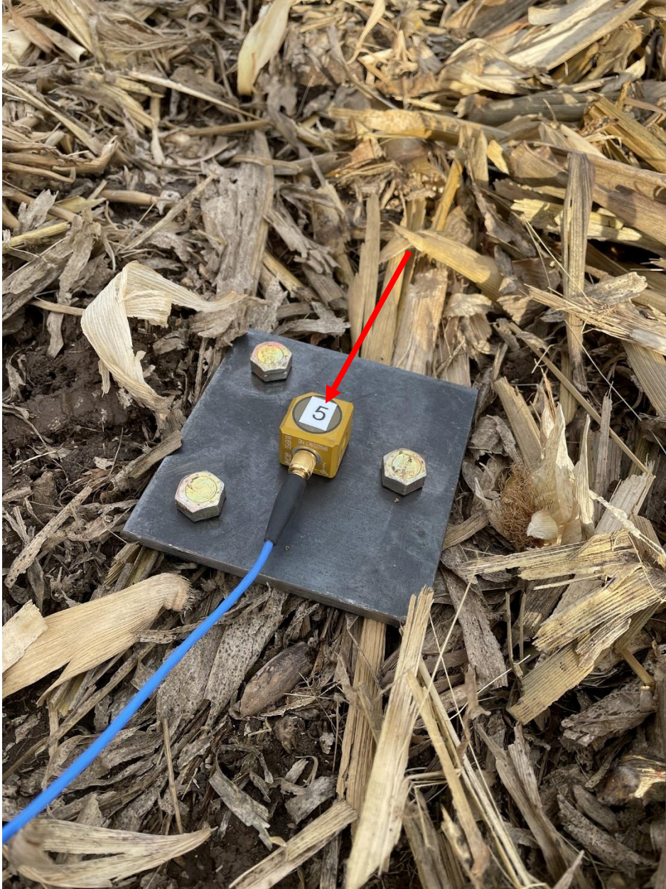
Figure 5. Typical accelerometer installation without cover. Sensor indicated by red arrow.
