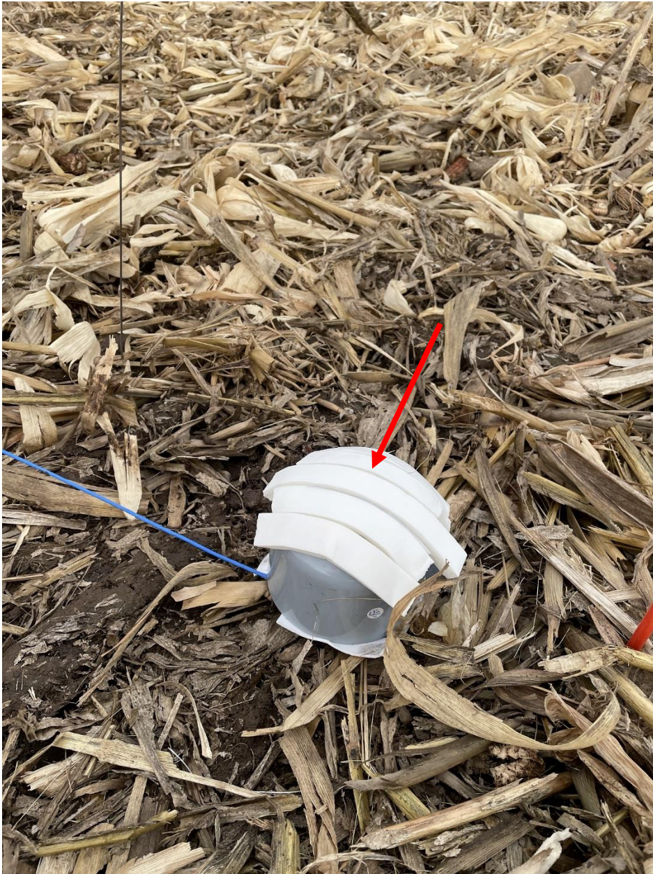
Figure 6. Typical accelerometer installation with cover (red arrow).
